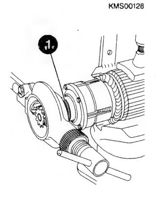
Checking needle bushing in armature
